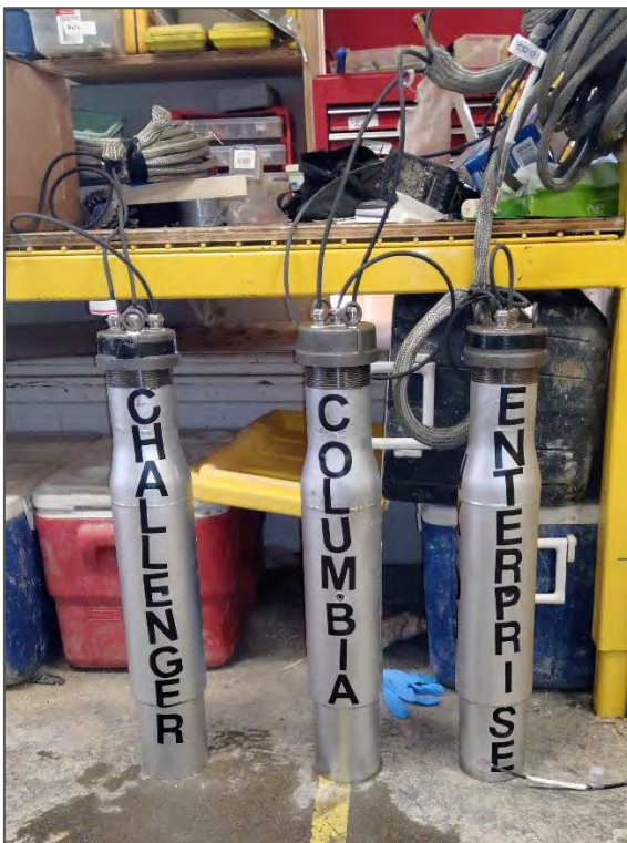
Photograph 3: Assembled protective steel casings containing sets of accelerometers (3 orthogonal directions); Installation of protective steel casing containing a set of accelerometers (3 orthogonal directions) (right)
