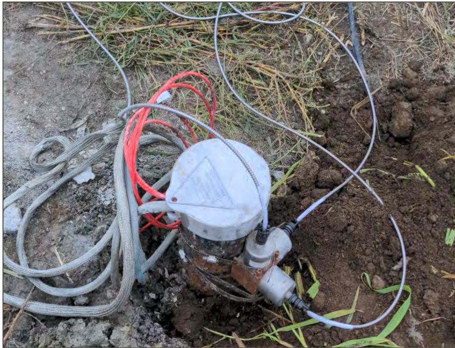
Photograph 4: One set of accelerometers (3 orthogonal directions) mounted on one mock well at ground surface.
