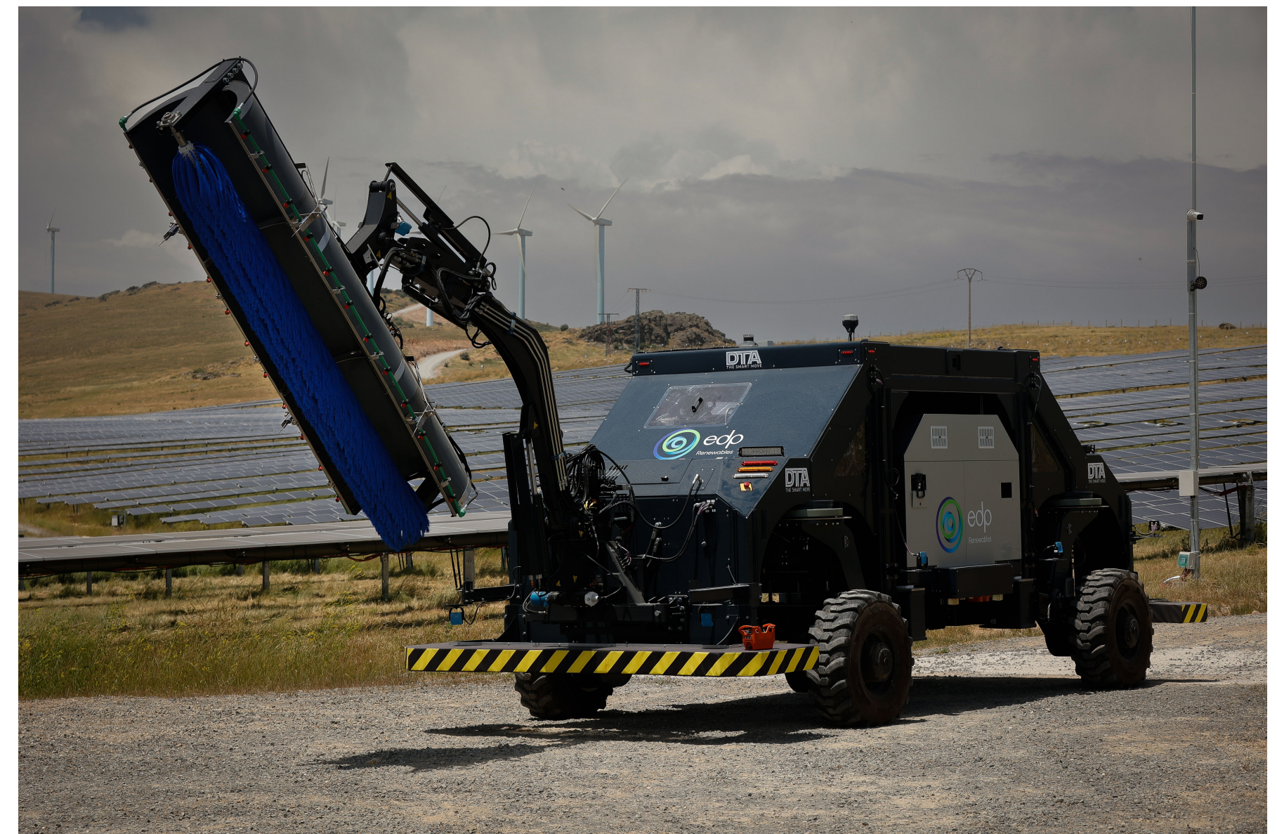
Image: Scale up O&M – Autonomous robotic cleaning solution for utility-scale solar parks, improving photovoltaic panel performance, reducing maintenance needs, and supporting more efficient renewable energy generation.
