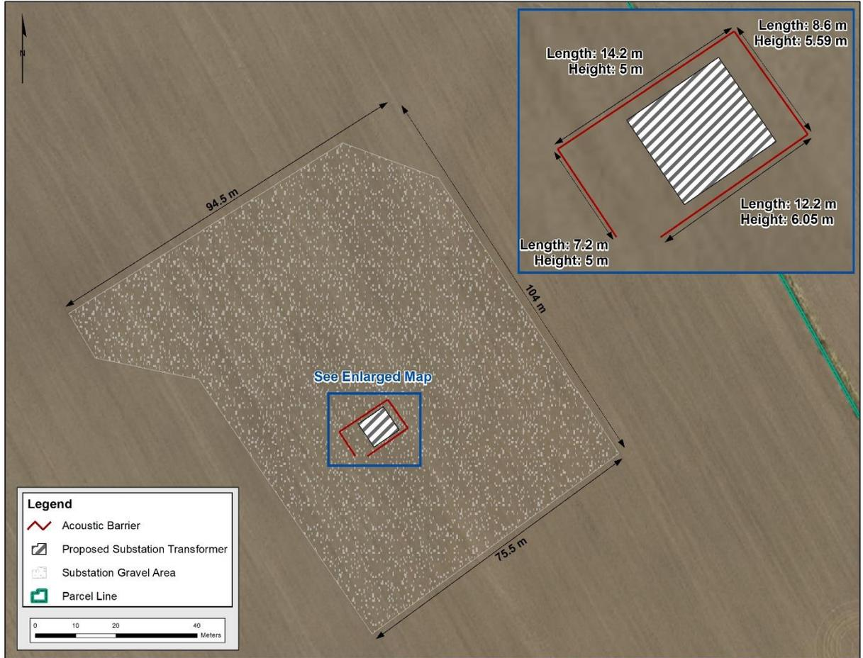
**Figure 4-1 Project acoustic barrier and gravel area dimensions**
